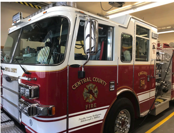
Engine 34 | Pierce Dash model year 2019 Carries 680 gallons of water and 20 gallons of universal biodegradable foam
