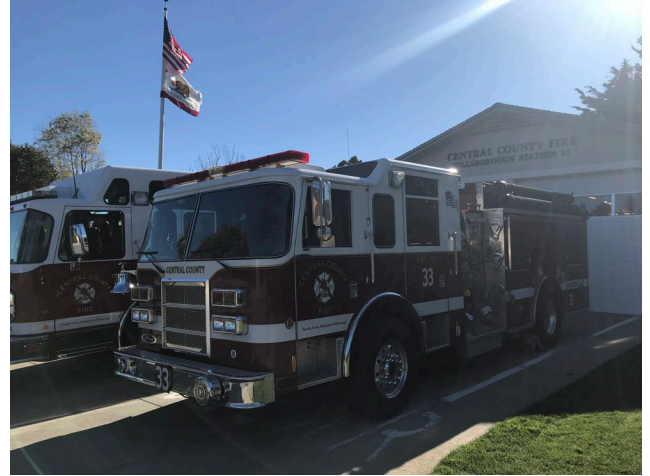
Engine 33 | Pierce Dash model year 2003 Carries 500 gallons of water and 20 gallons each of Class A and Class B foam
