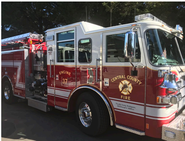
Engine 37 | Pierce Dash model year 2016 Carries 680 gallons of water and 20 gallons of universal biodegradable foam
