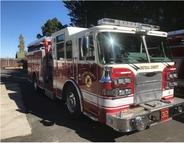
Engine 32 | Pierce Dash model year 2016 Carries 680 gallons of water and 20 gallons of universal biodegradable foam
