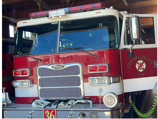
Engine 36 | Pierce Dash model year 2016 Carries 680 gallons of water and 20 gallons of universal biodegradable foam
