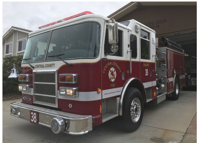
Engine 38 | Pierce Dash model year 2017 Carries 680 gallons of water and 20 gallons of universal biodegradable foam
